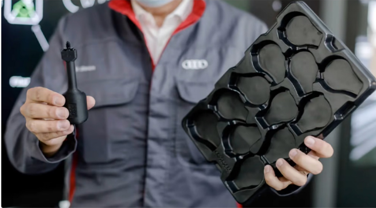
A technician at Audi holds up a manufacturing tool and the plastic packing waste it was 3D printed from. (Source: Audi)
